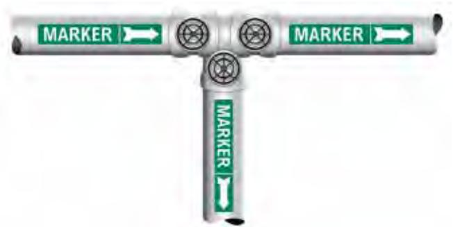
Install pipe labels close to valves or flanges
