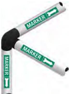
Install pipe labels near branches and whenever a pipe changes direction.
