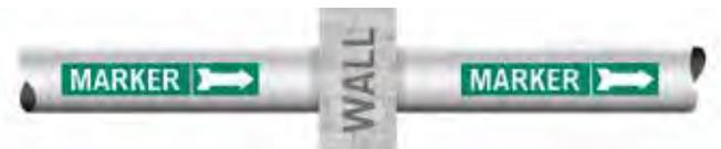
Install pipe labels before and after all wall, floor and ceiling penetrations.
